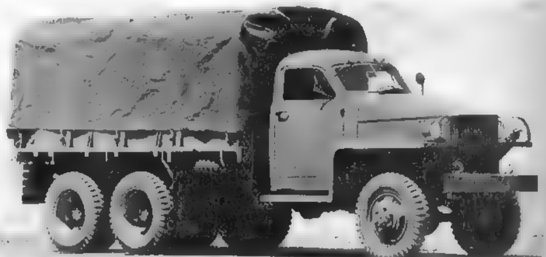
While the final US6 trucks had metal-enclosed cabs, the beds were made of wood. (U.S. Army photo).
